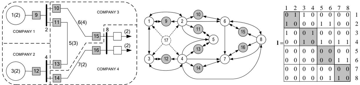
Figure 1 – Graph and Forced Adjacency Matrix of Typical Electrical Power Grid
